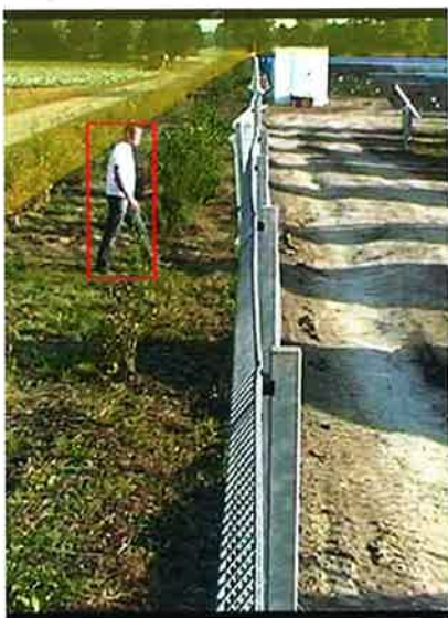
▲ Analytics can be deployed at perimeters, to detect unauthorized intrusion. (Image courtesy of Viysis Intelligent Video)
